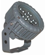
MODEL: GA-FCR9 FACADE LIGHT: 9W LED COLOR: WW/CW/NW/R/G/B DIMENSION: 130x90mm BEAM ANGLE: 24,36,48deg IP:66 BODY COLOR: Gray
