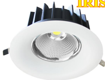
MODEL: GASP-0202 SPOT LIGHT: 7W/12W/18W LED DIMENSION: 85x40/110X52/140X65mm CUTOUT SIZE: 65/90/115mm NON-MOVABLE LIGHTS
